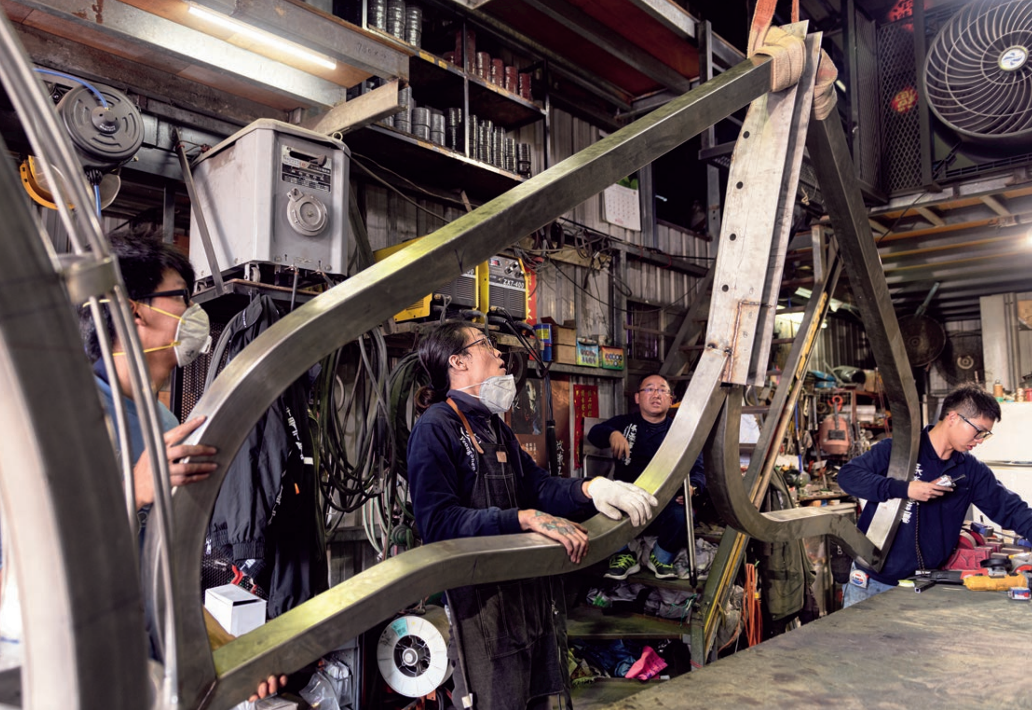
Zeng Wen-chang and employees in his ironworks shop work on a bus stop shelter in the shape of a whale tail (left). A young worker welds components of the bus stop shelter (above).
