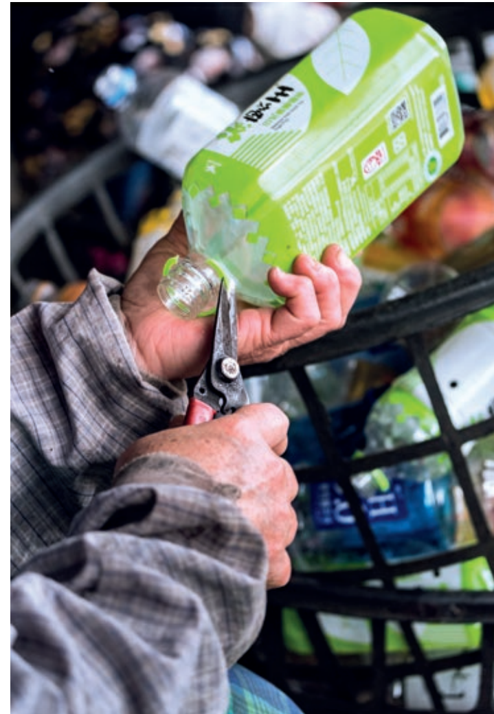
A volunteer removes the ring from the neck of a PET bottle. The ring and cap of a PET bottle are made of a different material from the bottle itself. They need to be removed and recycled separately.
